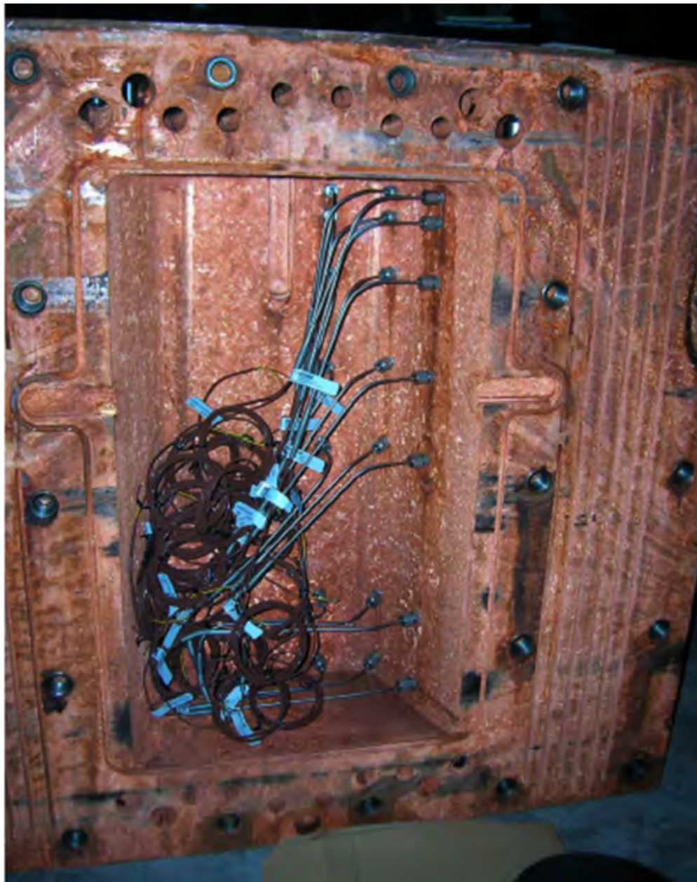
Figure 2.3 Back of the beam-blank mold instrumented with 47 thermocouples
